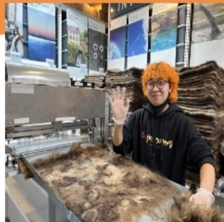
Lonnie filling 2 scrims with short fibers 1-4" (3-10cm)
