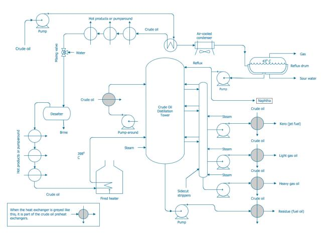
One of the fractions, naphtha, is an important component used to massproduce plastic. Naphtha decomposes at a high temperature (1,472° F / 800° C) to produce aromatics (e.g., toluene, benzene, and xylene) and olefins (e.g., ethylene [2 carbons], propylene [3 carbons], butane, butadiene, and butylene [4 carbons]). These are all monomers, the building blocks for polymers when monomers are put together through chemical bonds.
