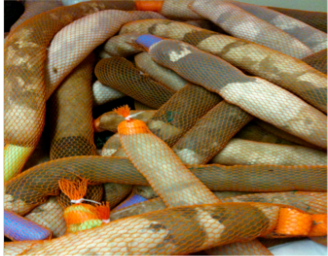
Multiple hair booms inside industrial netting with piece of pool noodles added to make them float. The use of pool noodles is another example of a synthetic material being used with the natural materials.
